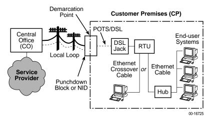
DSL - Digital Subscriber Line NID - Network Interface Device ----- New Wiring Connections
